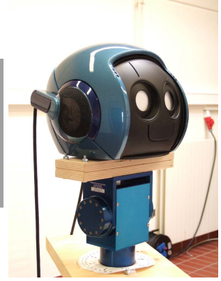
Fig. 6. Left: Bionic ears used in our system. The ears are modeled after the human outer ears. The blue line indicates the concha of the left ear, while the white one corresponds to the right ear's concha outline. Right: Our robot head with two human-like ears on both sides mounted on a pan-tilt element.
